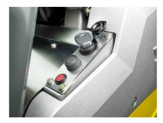
Simply start the DPU 4045 with an ignition key. A loud signal tone prevents inadvertent draining of the battery.
